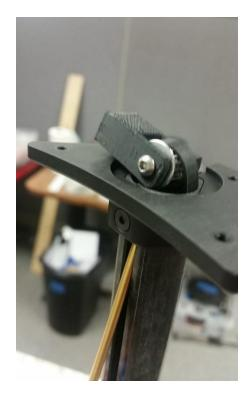
• Now remove the screw holding the pulley in place. (be sure not to drop anything into the rod and to not twist or re-orient the belt)
