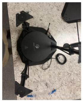
• On the base of the printer near the bottom of each rod is a hole whereby the pulley and belt can be accessed by two fingers, pictured below. Make a mental note of how tight the belt is on the pulley by squeezing both sides between your thumb and pointer finger. Upon reassembly you will need to tighten the belt to this same amount of tension
